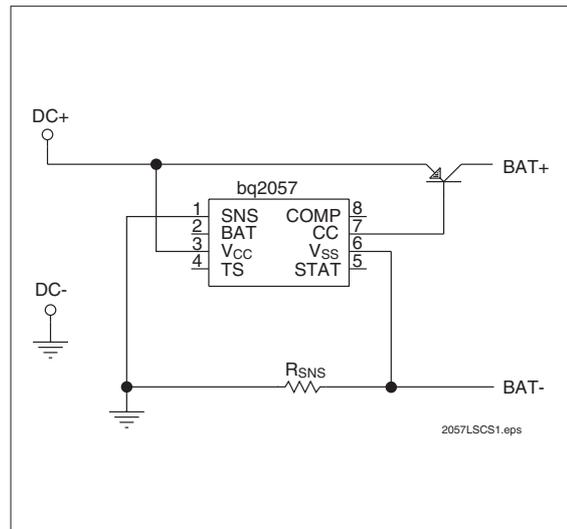
Figure 6. Low-Side Current Sensing
