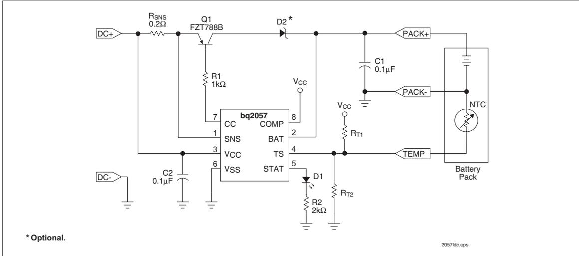
**Figure 3. Low-Dropout Single- or Dual-Cell Li-Ion Charger**
