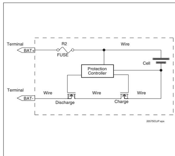
Figure 11. Typical Components of a Single-Cell Li-Ion Pack
