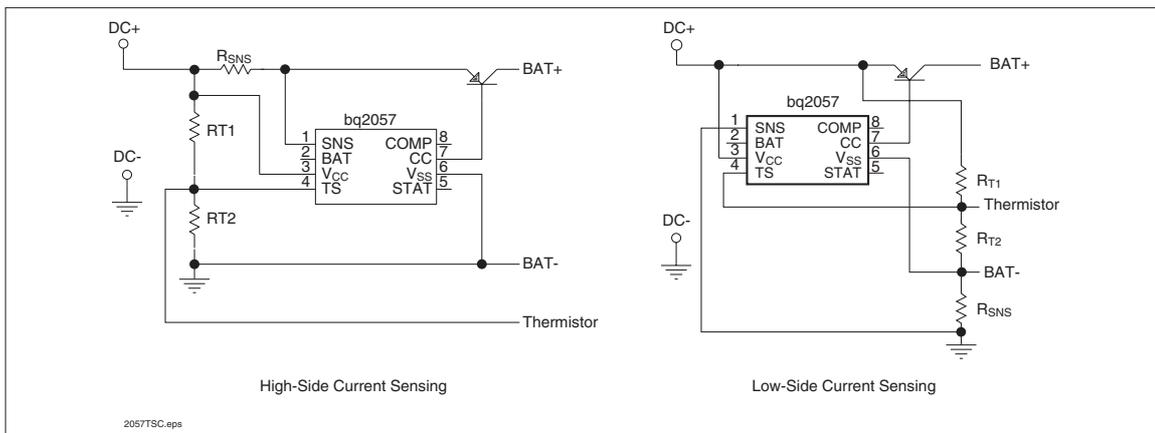
**Figure 9. Temperature Sensing Circuits**
