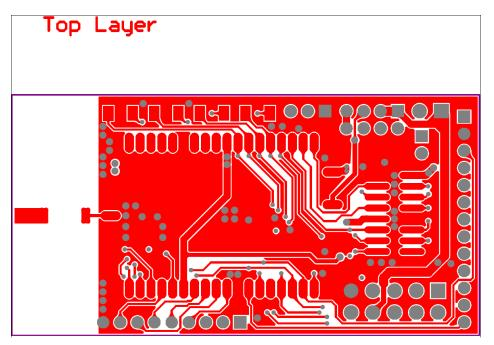
The feed connecting the antenna to the RF pad has to be 50ohm in impedance. If this feed is shorter than 0.2" the board can be a 2 layer and the thickness of the feed is the same as described in the manufacturer's datasheet. If the trace is longer than you need a 4 layer board, with controlled impedance. That means a ground plane directly under the top layer. The thickness should be calculated accordingly.
