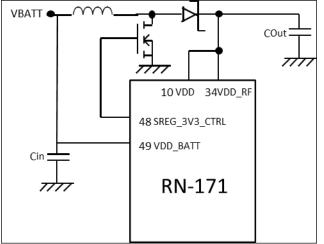
Designs that include the boost regulator will provide good supply to the flash even when the battery voltage drops close to 1.8V.
