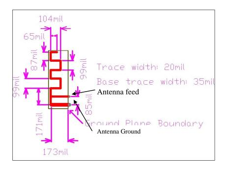
The trace form the RF pad to the antenna feed should be of 12mil thickness on a four layer PCB to achieve 50 ohms impedance matching. This is shown in the diagram below:
