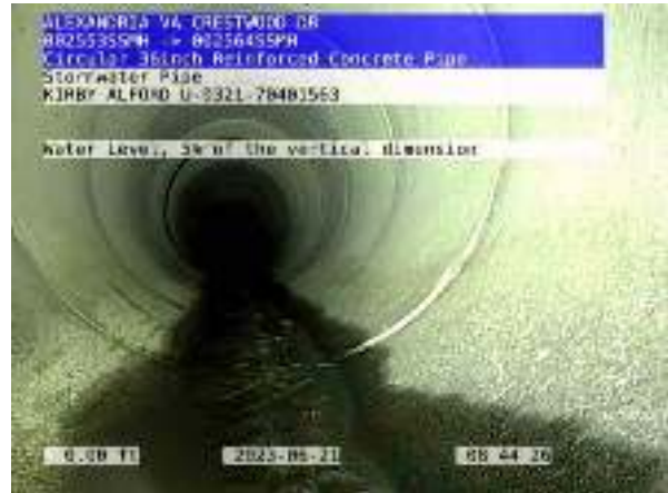
007464STMP_69e783d0-adf1-48ce-bda1-ad6928900325_202 30621_091713_871.jpg, 00:00:15, 0.00ft Water Level, 5% of the vertical dimension
