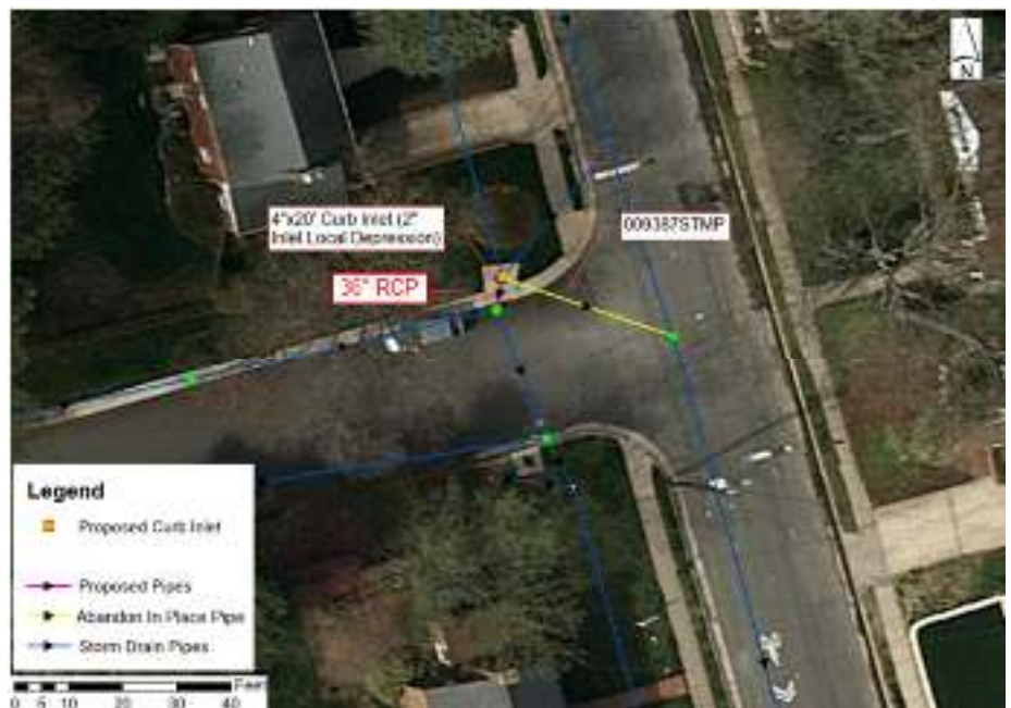
Figure 10: Dogwood Drive Storm Drain Pipe Realignment
