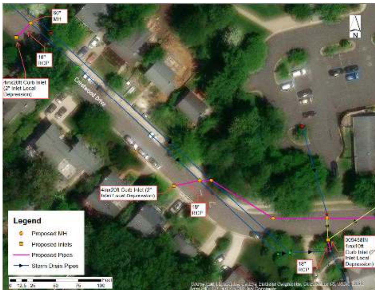
Figure 8: Proposed Curb Inlets along Crestwood Drive
