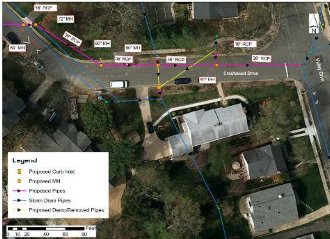
Figure 7: Proposed Storm Drain System along Crestwood Drive
