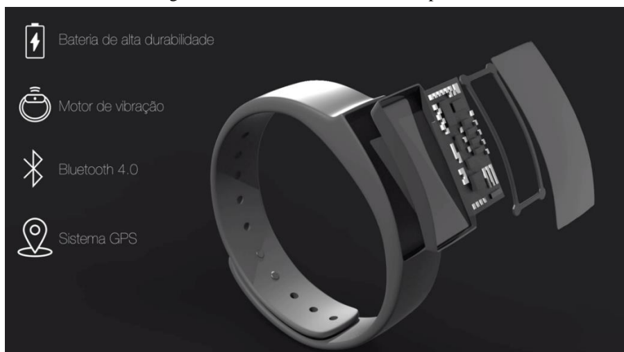
Figura 83 – Pulseira Silence, vista explodida
