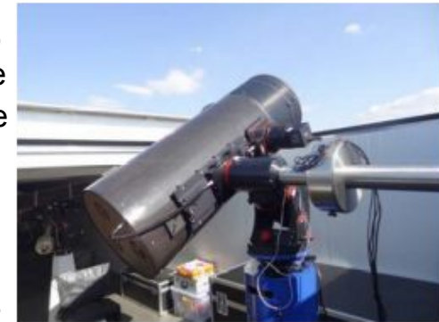
Airbus Robotic Telescope (ART) is Airbus' own end to end capability for Space Surveillance & Tracking, performing automated optical observations of space objects from LEO to GEO.
