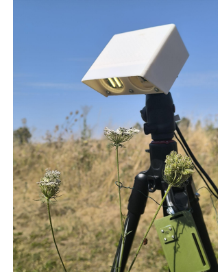
An “Entomoscope”, a device to monitor pollinators
