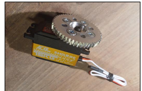
Figure 18: Steering servo + wheel
