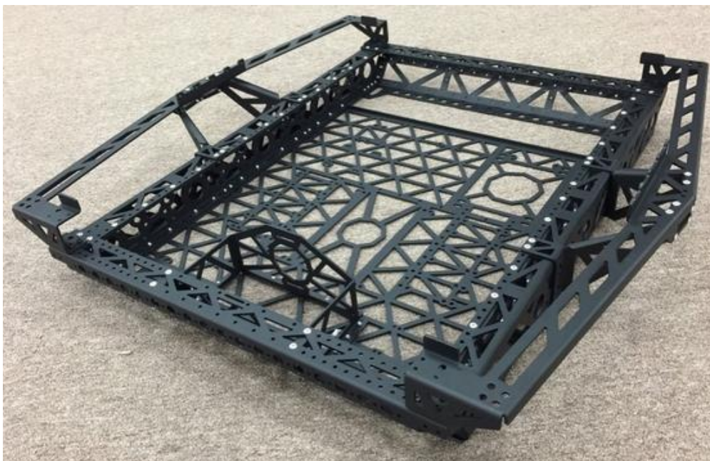
Figure 3.36: An FRC (FIRST Robotics Competition) chassis made from riveted sheet metal.
