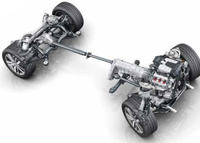
Figure 8.24: Drivetrain of a car
