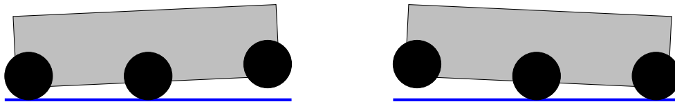
Figure 8.28: Side view of dropped-center drivetrain rocking fore-aft. Center drop is exaggerated.
