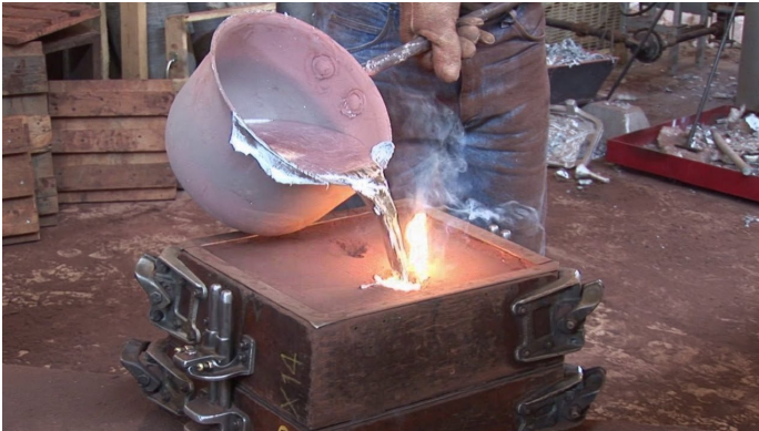
Figure 3.4: Left: the casting process. Right: A cast differential housing.
