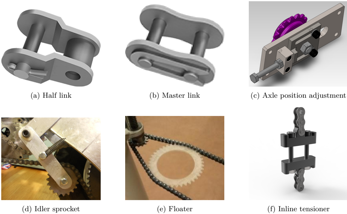
Figure 4.13: Various different adjustment methods for chain.
