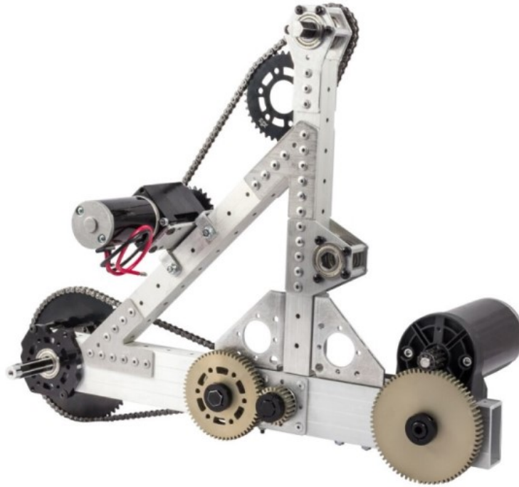
Figure 3.38: Tubes held together with sheet metal gussets.
