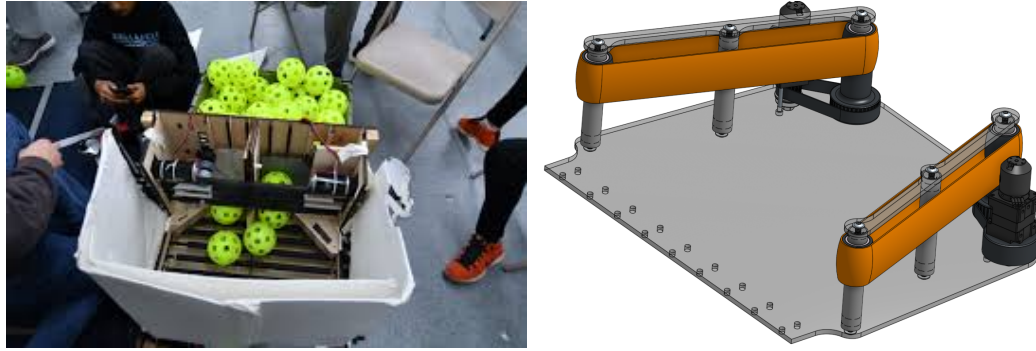
Figure 8.10: Agitated hoppers.
