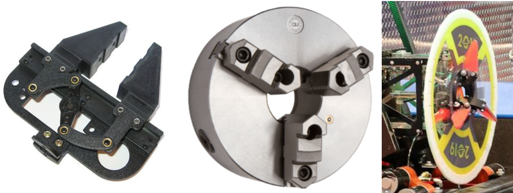
Figure 8.1: Jaw-based grippers.
