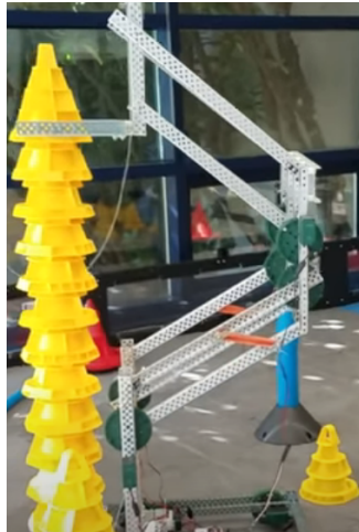
Figure 8.18: Double-reverse 4 bar.
