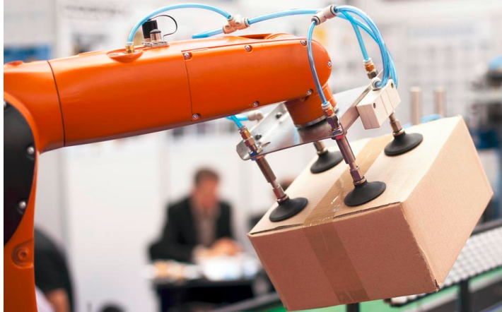
Figure 8.6: Vacuum gripper on a robot arm lifting a cardboard box.
