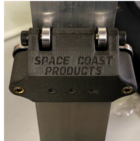
(e) Elevator bearing assembly
