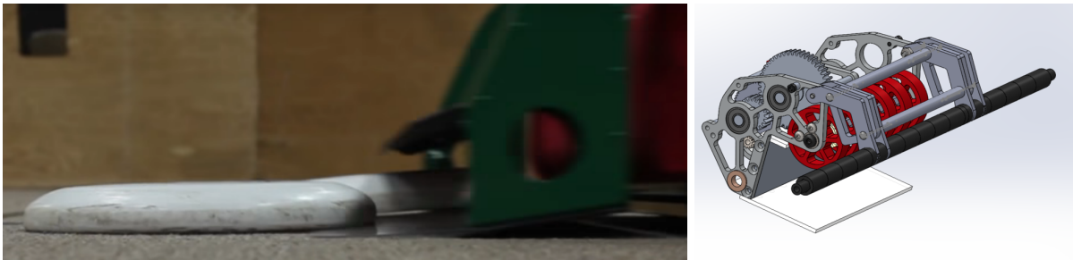
Figure 8.5: Left: scoop picking up frisbees. Right: scoop with additional beater bar (in red).
