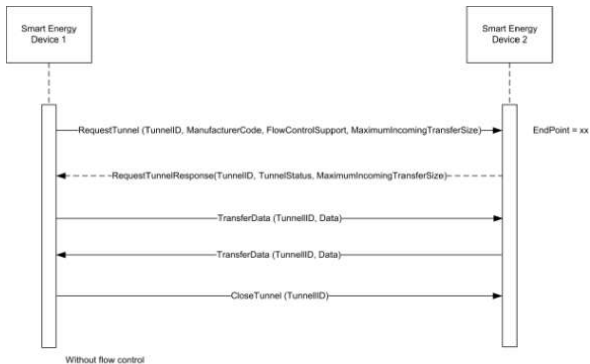
Figure 10-42. SE Device 1 (Client) Requests a Tunnel from SE Device 2 (Server) to Transfer Data Without Flow Control (Default)
