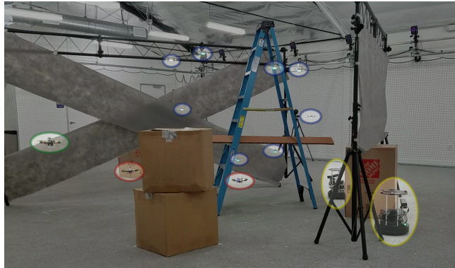
Fig. 1. A robot team with 10 small UAVs (blue, 8 visible), 2 medium UAVs (red), 1 large UAV (green), and 2 ground robots (yellow) is tasked with navigating a cluttered environment.
