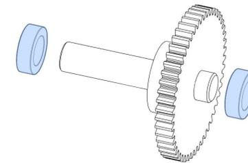
Remove the bearings from the shaft after checking the fit and continue with the assembly.
