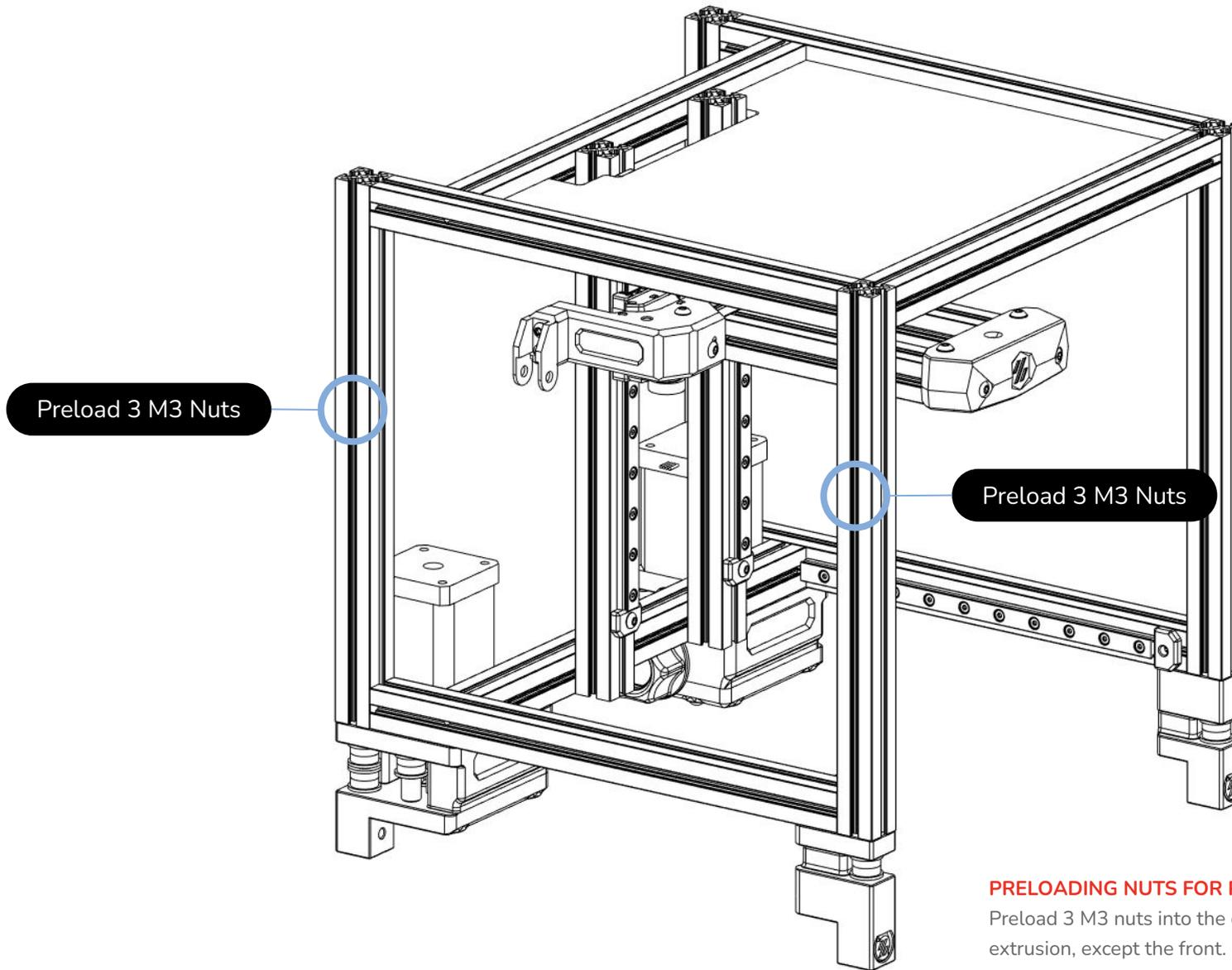
**PRELOADING NUTS FOR PANEL CLIPS**
