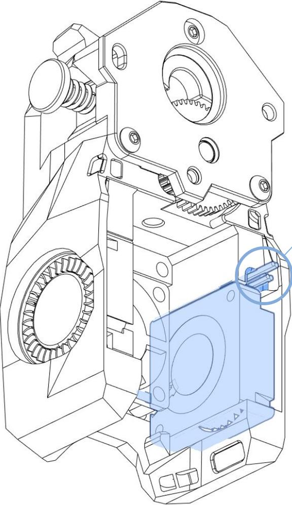
Guide the wires in the highlighted path.
