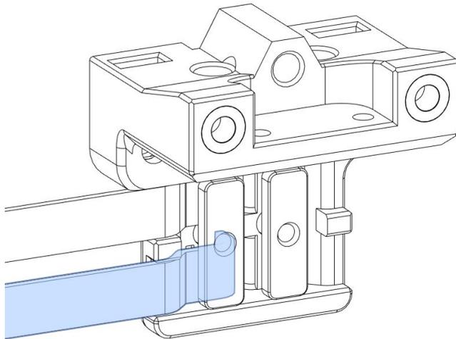
**Before** we run the belts, make sure your tensioner knobs are as loose as possible and your motors are as far to the outside of the printer as they can be.
