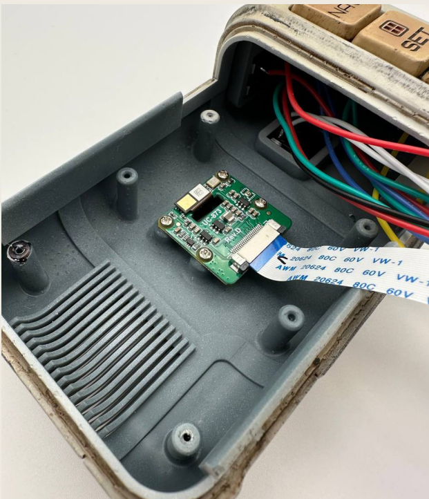
FIG. 06-12 – IMX519 camera module screwed to the bosses inside the front shell, CSI ribbon attached before mounting.
