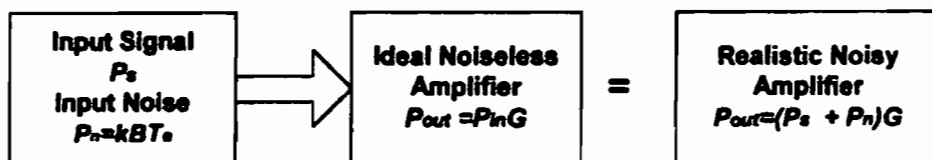
Fig. 9.15 Representation of noisy amplifier.
