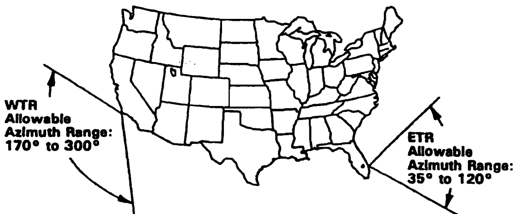
Fig. 3.27 Acceptable launch azimuth range for the United States.
