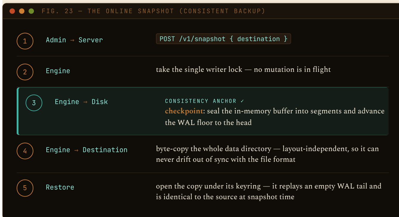
FIG. 23 — Consistency comes from the checkpoint plus the single-writer lock; the copy itself never parses a segment, so it captures new artifacts for free. The crash gate is untouched.
