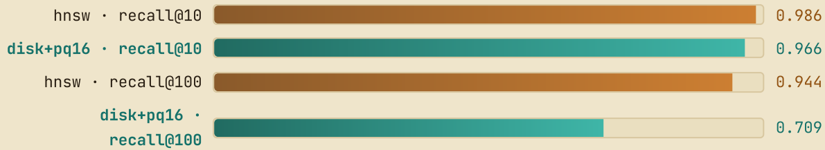
FIG. 20 – Compression keeps the head (recall@10 barely moves) but trades the tail (recall@100 collapses). The serving-RAM number is reference-hardware-pending on the shared dev box: post-build RSS here is the build’s allocator high-water mark, while the representative figure is the cold-reopen footprint where only the PQ codes (plus the small delta and codebook) stay resident – the metric the durable disk index (ADR-0063) finally makes real and the wedge runner now samples after a cold restart. So it is omitted, not estimated.
