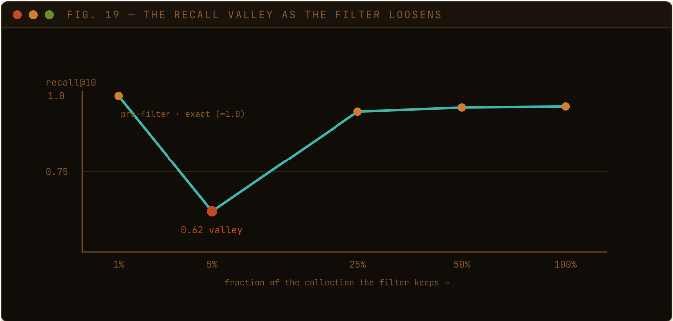
FIG. 19 – Always correct, never wrong: the filter is re-checked on every survivor (§4.5), so the “valley” is a recall dip the planner trades for speed, not an incorrect answer. Very selective filters pay in scan latency instead.
