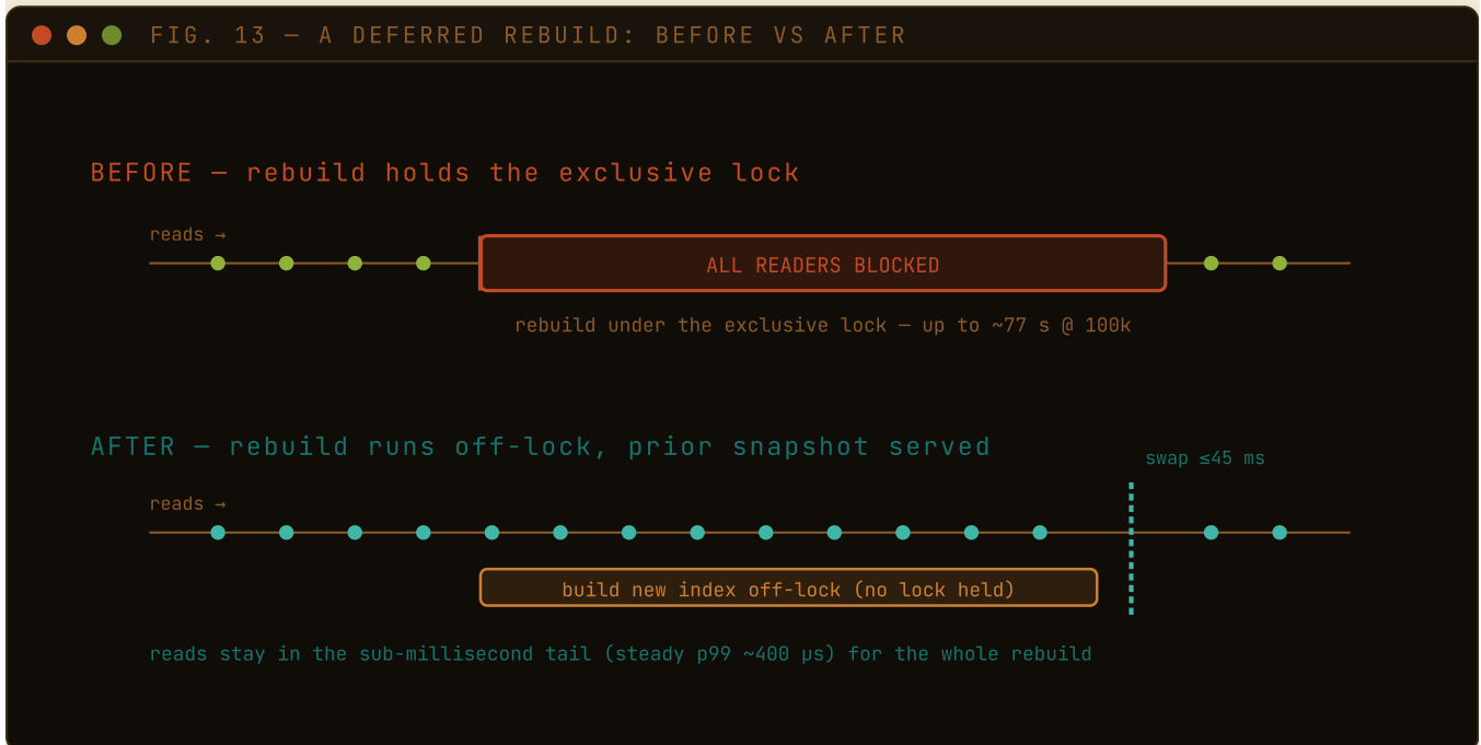
FIG. 13 – The seconds-long stall (top) collapses to the cost of serving the prior snapshot plus a brief swap (bottom). No unsafe , no lock-free data structure – just Arc and the existing RwLock .
