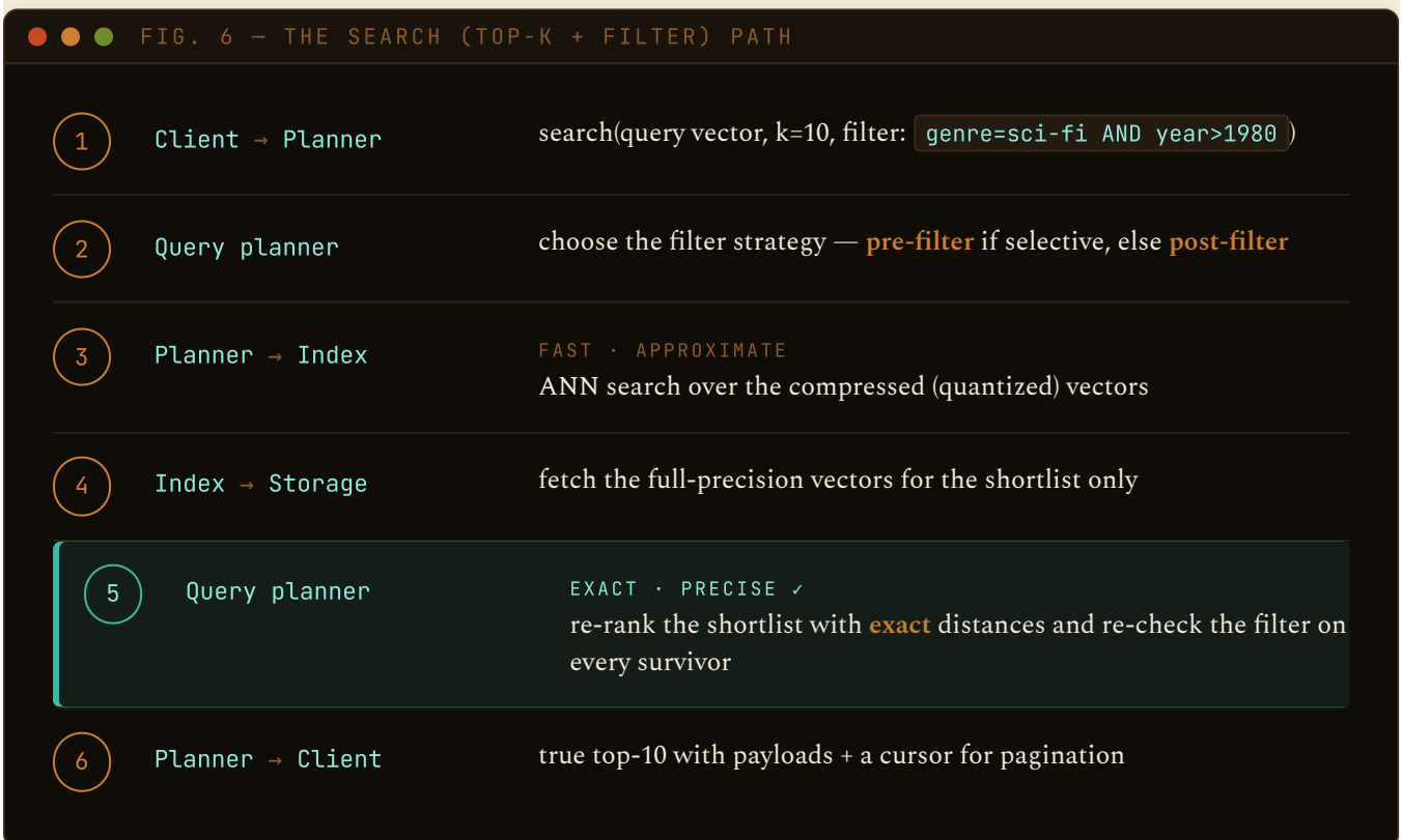
FIG. 6 — The two-phase pattern: cheap approximate narrowing, then exact precision on the shortlist.
