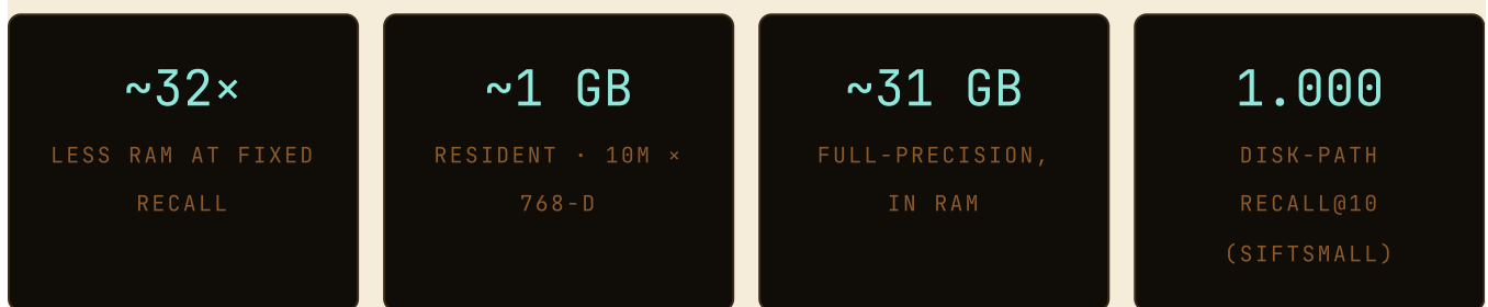
FIG. 21 – On SIFTSMALL the disk path serves recall@10 up to 1.000 while holding only PQ codes in RAM. The head-to-head RSS vs Qdrant/LanceDB is explicitly reference-hardware-pending – never fabricated.
