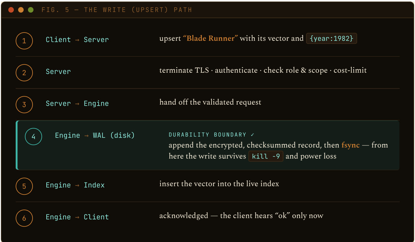
FIG. 5 — The write is acknowledged only after the record is physically on disk.
