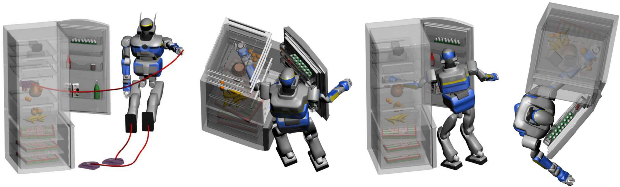
Fig. 10. Pick-can-from-fridge scenario. From left to right: illustration of the target, posture obtained without collision avoidance constraints, successful free-collision posture found (side and up views).
