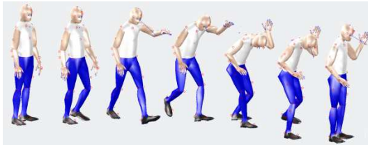
Figure 3: Snapshots of a reconstructed motion: passing under a beam (not represented) with left hand grasp.
