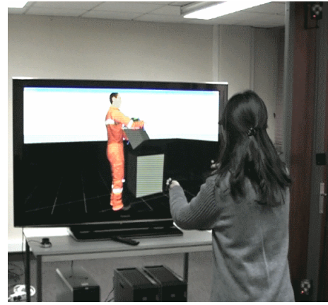
Fig. 1. Real-time manipulation task control based on motion capture. The markers are attached on the hands of the operator.
