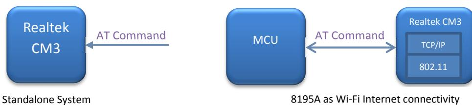
Realtek CM3 attaches to MCU through UART or SPI, and MCU control Realtek CM3 through AT command.
