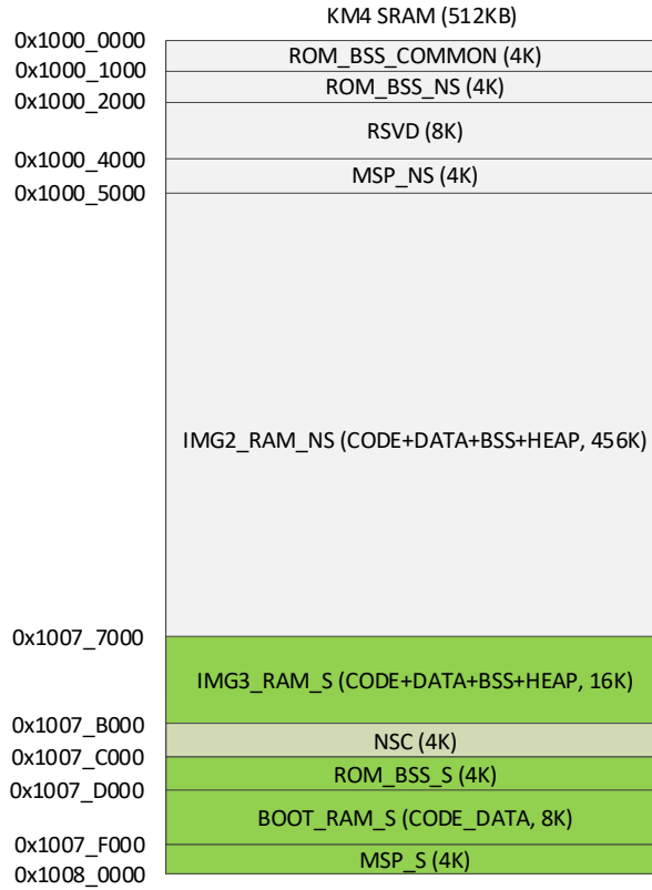
Fig 9-5 KM4 RAM program layout
