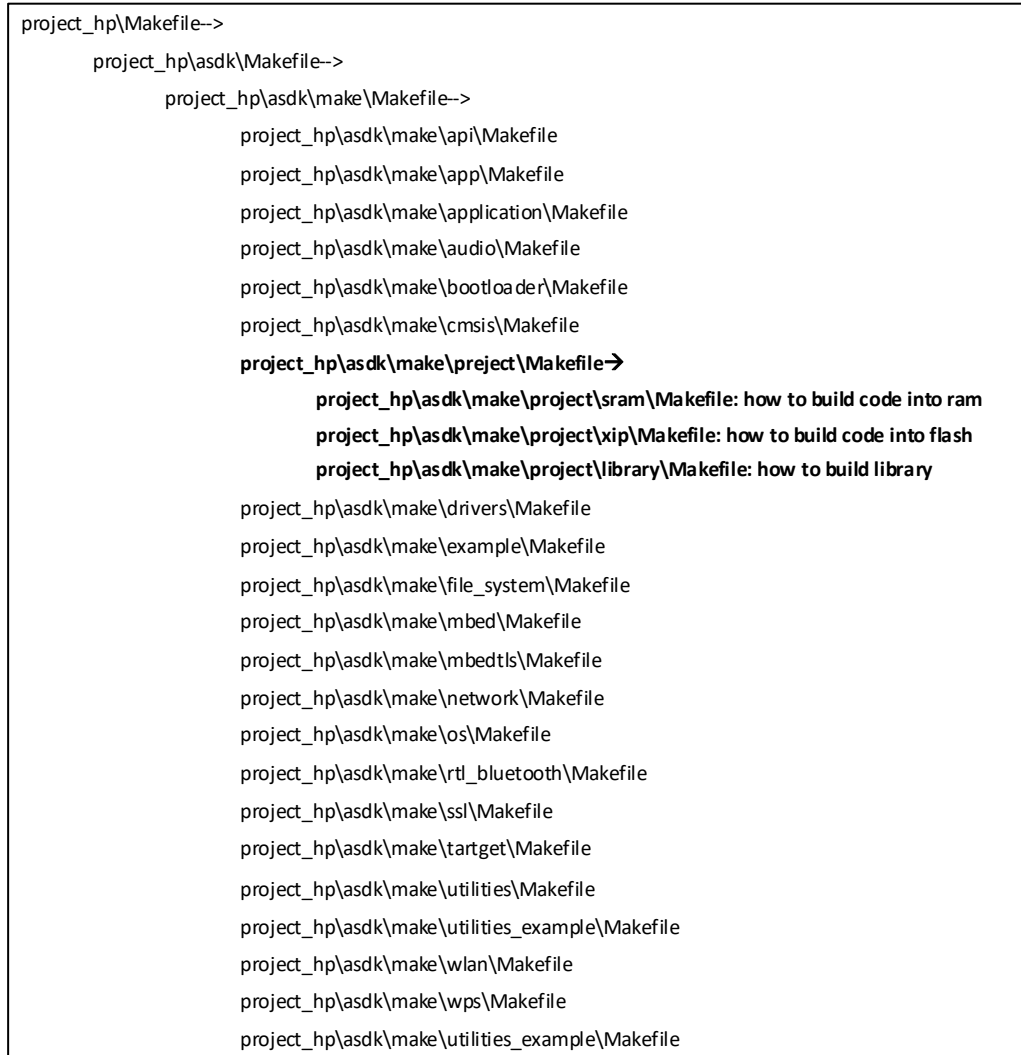
Fig 3-1 KM4 Makefile architecture
