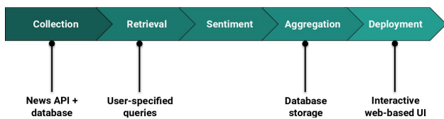
Figure 10: Layout of end-to-end pipeline
