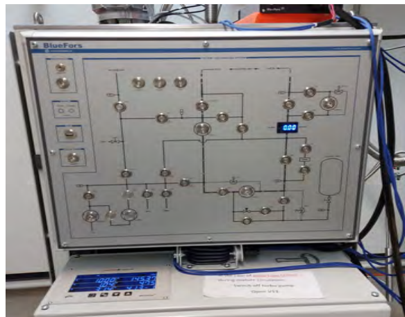
(d) The control station of the cryostat, which is responsible for cooling the TES.
