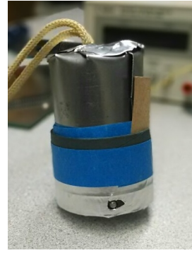
(a) Automated taper with solenoid head visible.
