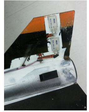
(b) Detail of strain gauges 12 and 13, mounted to a fin
