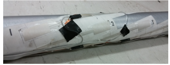
(c) Strain gauges 1, 2, and 3. Gauge 11 (orthogonal gauge) is partially visible above gauge 2
