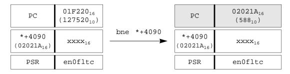
4. Passes execution control to a non-sequential instruction if the PSR.Z flag is 0. The instruction passes execution control by adding 1507344 to the PC register.
