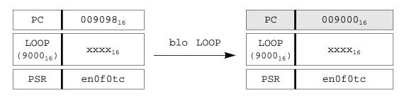
2. Passes execution control to a non-sequential instruction if the PSR.Z flag is 0. The instruction passes execution control by adding 16 to the PC register.
