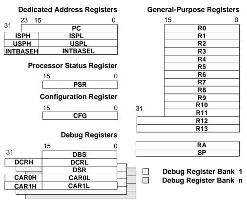
The number of debug registers depends on the configuration of the chip
