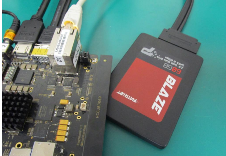
Figure 33 - Plug in eSATA cable and SSD
