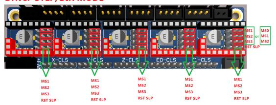
Note: if you are using A4988 or DRV8825 driver, you must connect RST and SLP with jumper cap.
