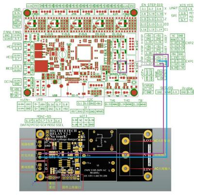
6. The connection of SKR V1.4 and Resume Printing While Power Off Module (UPS 24V V1.0) :
