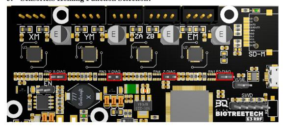
Use the jumper to connect the corresponding axis as shown in the figure to use the Sensorless homing function;
