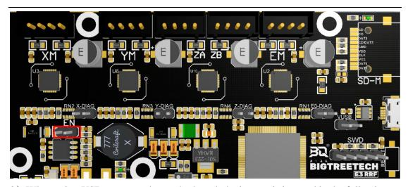
$2)\,$  When using USB to power the motherboard: the jumper is inserted in the following "VUSB" position
