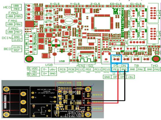
6. The connection between BIGTREETECH SKR 2 and power failure (UPS 24V V1.0):
