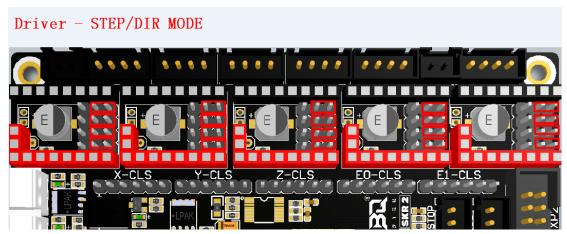
Note: If you use A4988 or DRV8825 driver, you must short-circuit RST and SLP with a jumper cap to work normally.
