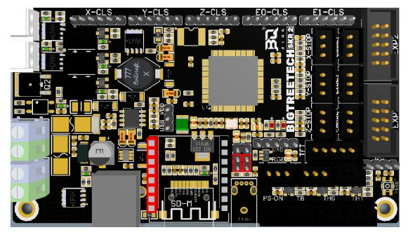
②RRF WIFI function: If selected (as per the jumper configuration below), the U disk function will not be available as WIFI will work through SPI mode, and RRF firmware can be used.
