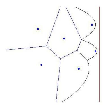
When a site is no longer associated with active arcs of the beachline its Vornoi cell has been completed
