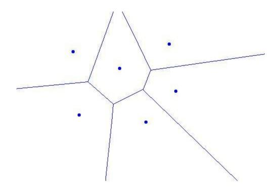
Voronoi edges on the periphery of the diagram extend to infinity
