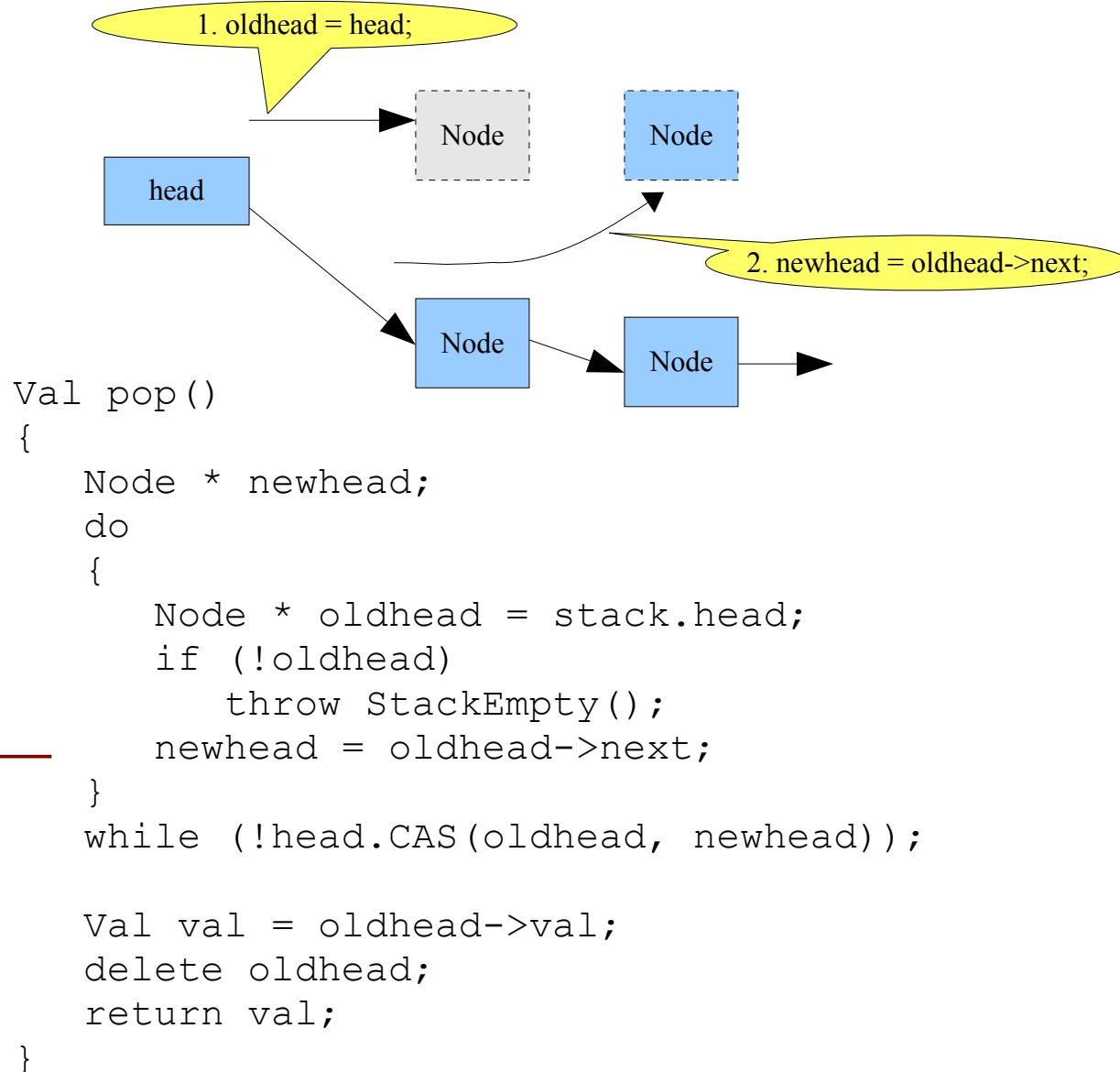
*ABA – ...And then reused (recycled by Allocator) and Pushed:*
