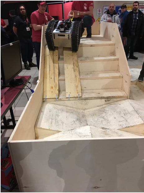
Fig. 4. Picture of our small scale test method – This test method is 8'x12' and is used to test the following cases: stairs, parallel rails, step-fields, and inclined plane
