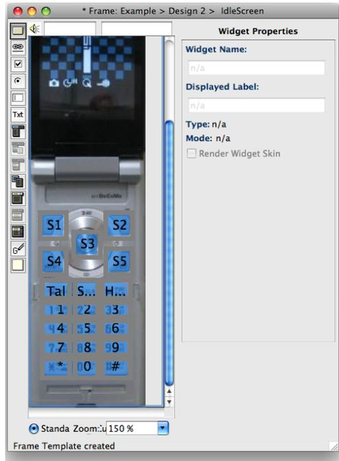
Figure 4-16: All the Widgets that represent the hard keys on this cellphone have been selected and, from the Modify menu, the designer has chosen Set Frame Template. This is indicated in the status message at the bottom left of the window, which reads: “Frame Template created”. Each time a new Frame is created in this Design, it will already have these buttons in it.
