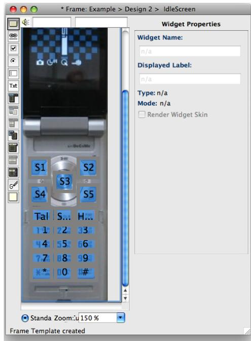
Figure 4-12: All the Widgets that represent the hard keys on this cellphone have been selected and, from the Modify menu, the designer has chosen Set Frame Template. This is indicated in the status message at the bottom left of the window, which reads: “Frame Template created”. Each time a new Frame is created in this Design, it will already have these buttons in it.
