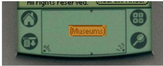
Figure 4-15: The Museum button has been captured for the Widget from the upper right of the Frame background. The Widget has been moved to the Graffiti area (a silly thing to do) to illustrate how the captured image looks.
