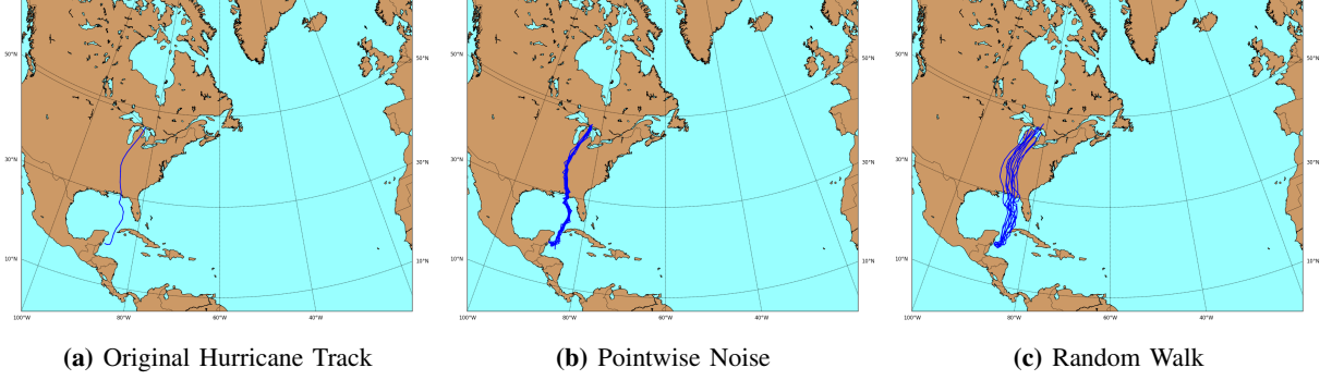
Fig. 6: A comparison of the impact of adding noise to copies of the track of a single hurricane with the pointwise noise method and the random walk method. The random walk clearly is more desirable, as it both appears smoother, and has greater variance.
