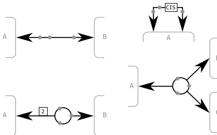
**Figure 2.19:** *The Entity Relationship glyph for interaction. Top left, binary interaction between two entities. The circle can be omitted, and the outcomes located anywhere on the interaction. Bottom left, because the cardinality of the entity A is 2, the interaction is not a binary one, but a n-ary one. The circle cannot be omitted. Bottom right, n-ary interaction with three different entities. Top right, intra-molecular interaction;*
