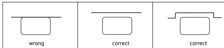
**Figure 4.3:** Edges must not overlap node borders.
