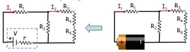
1) What is I<sub>1</sub>, the current that flows through the resistor R<sub>1</sub>?
