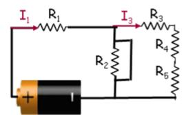
Resistor R<sub>2</sub> is now shorted out as shown. How does the magnitude of the voltage across the battery change?
