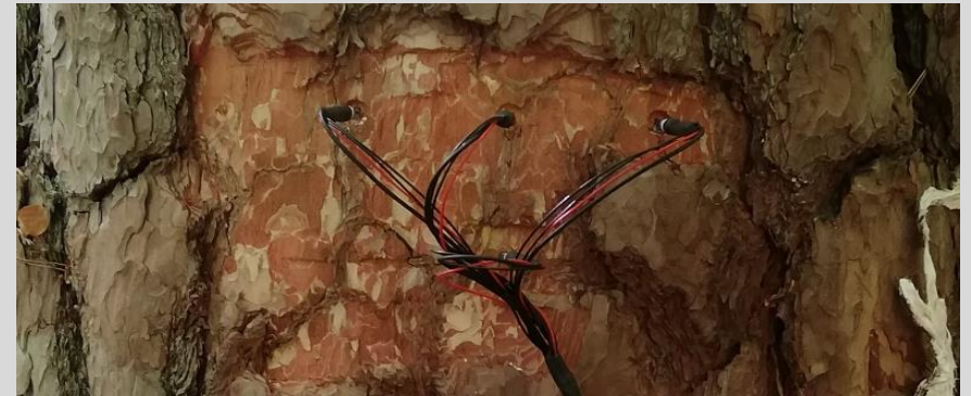
Fig. Examples of an linear variable differential transformer (LVDT) dendrometer installed on a birch tree (top) and thermal dissipation probes (TDP) installed on a Scots pine (bottom), to measure stem radial change and sap flow, respectively.
