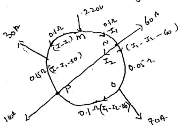
Let current in section mno be  $I_1$  and in section np be  $I_2$ .
