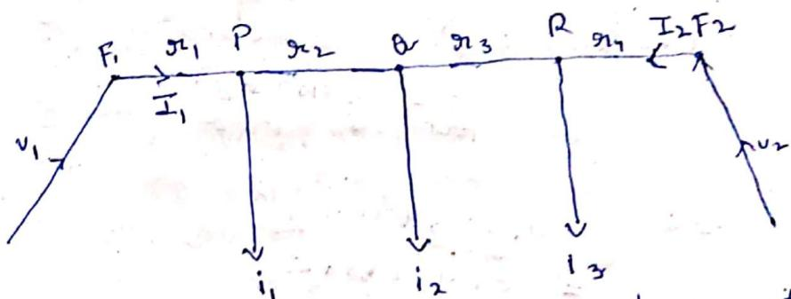
Consider a distributor fed at  $F_1$  and  $F_2$  with voltages  $v_1$  and  $v_2$  respectively as shown in fig.
