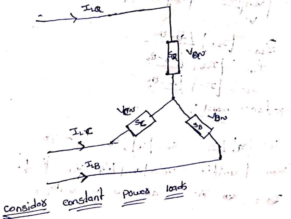
$$S_a = |S_a| \underline{L^{\theta_a}} \quad S_b = |S_b| \underline{L^{\theta_b}} \quad S_c = |S_c| \underline{L^{\theta_c}}$$
