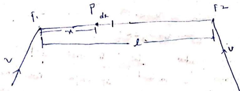
consider a point P on distributor at distance of  $x$  from feeding point "F1" as shown in above fig.
