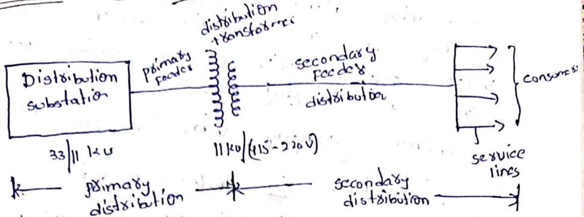
distribution system starts from distribution substation. distribution substation consist of a transformer which stepped down the voltage from 33 KV which comes from transmission line to 11 KV.
