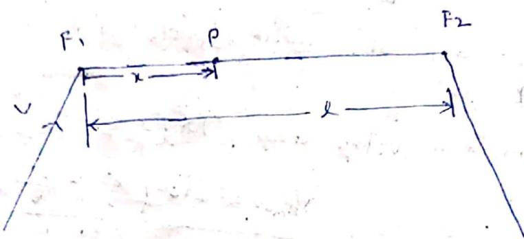
when the voltage at both ends is same, the middle point becomes the point of minimum potential. Thus the distributor can be image to be cut into two, at the middle point giving rise to two uniformly loaded distributors each fed at one end. The current applied to distributor is  $i_d$ .
