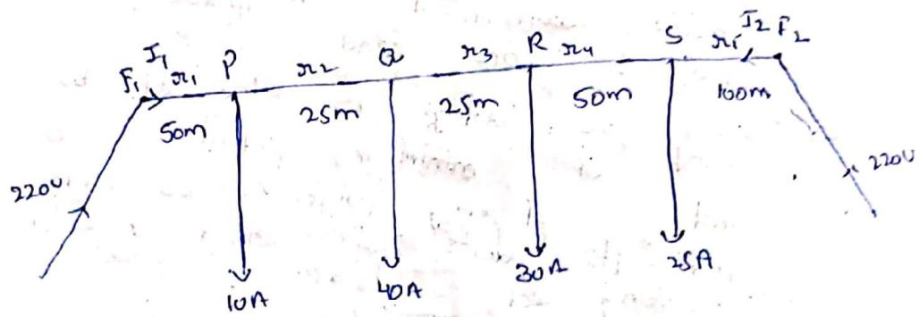
$$\text{Resistance/km} = 0.2 \Omega \\ = \frac{0.2}{1000} = 2 \times 10^{-4} \Omega/\text{m}$$
