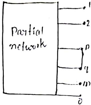
\* All the elements of the Bus Impedance Matrix must be recalculated to include the effect of the added link.
