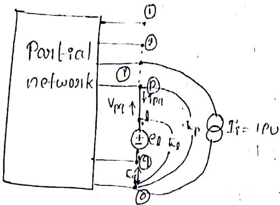
\* If the added element pq is the link then the procedure for recalculating the elements of the bus impedance matrix is to connect  $e_p$  in series with the added element.
