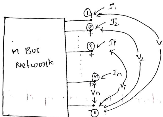
\* Figure shows a general n-bus linear passive network - the general form of the network performance equation. it is also an easy way to determine the  $Z_{\text{BUS}}$  matrix.
