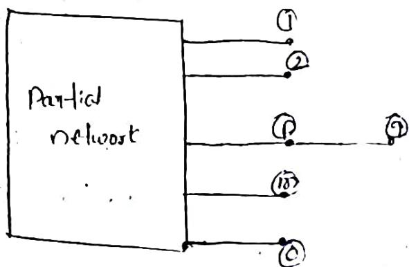
\* If  $PQ$  is a branch a new bus  $B_{PQ}$  is added to the partial network & the resultant  $Z_{\text{bus}}$  is of order  $(m+1) \times (m+1)$ .
