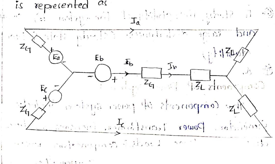
The 1- $\phi$  equivalent of balanced 3- $\phi$  work is as shown in figure
