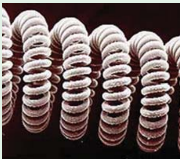
A electric filament is a metallic wire, usually made of tungsten, when heated to luminance by passing electricity, radiates light
