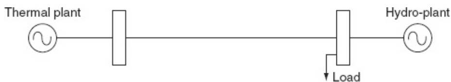
FIG. 6.4 A typical two-plant hydro-thermal system
