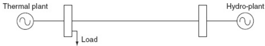
FIG. 6.3 A typical two-plant hydro-thermal system
