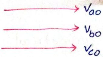
These phasors can be denoted by  $V_{a0}$ ,  $V_{b0}$  &  $V_{c0}$  as shown in fig.
