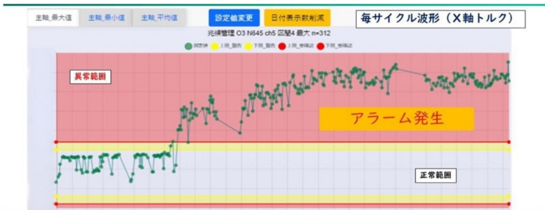
Spindle torque per cycle alarm on drift
