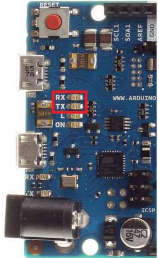
The pins are 3.3V and are **not** 5V tolerant. This port uses a software UART implementation which can be configured from 110 to 38400 baud.
