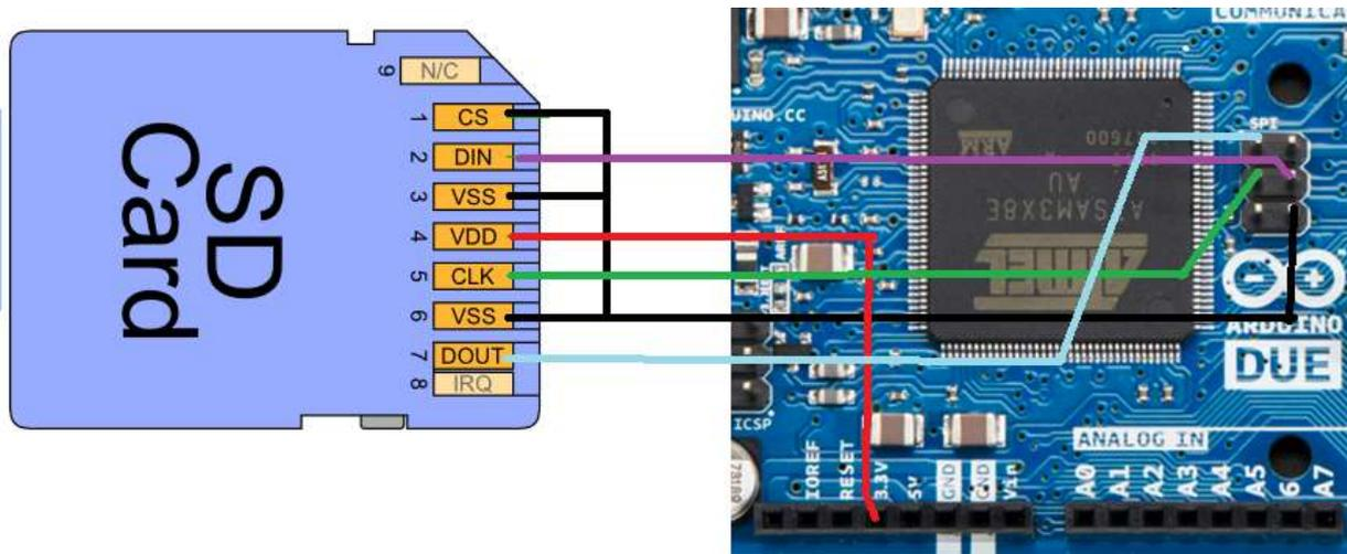
Unfortunately, there is no 3.3V pin on the SPI header on the Arduino Due so that wire must go to the (separate) 3.3V pin. Do not wire the 5V output from the SPI header to the card. Doing so could damage the SD card and/or the Due.
