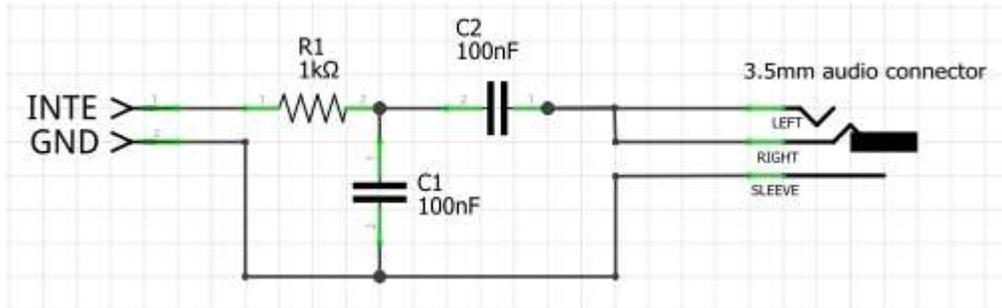
Connect the INTE input of the above schematic to the Arduino pin that drives the INTE light (pin D12 on the Due, pin D38 on the Mega) and GND to ground. The output is a line level mono signal that can be connected to the input of any amplified speaker system. It is not strong enough to drive headphones although but some mini earphones do produce a (not very loud) sound when plugged in.
