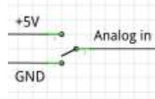
For the function switches we use the Arduino's internal pull-up resistors and just switch GND to the appropriate digital input. These are momentary SPDT (On)-Off-(On) switches. For example, the EXAMINE/EXAMINE NEXT switch is connected like this:
