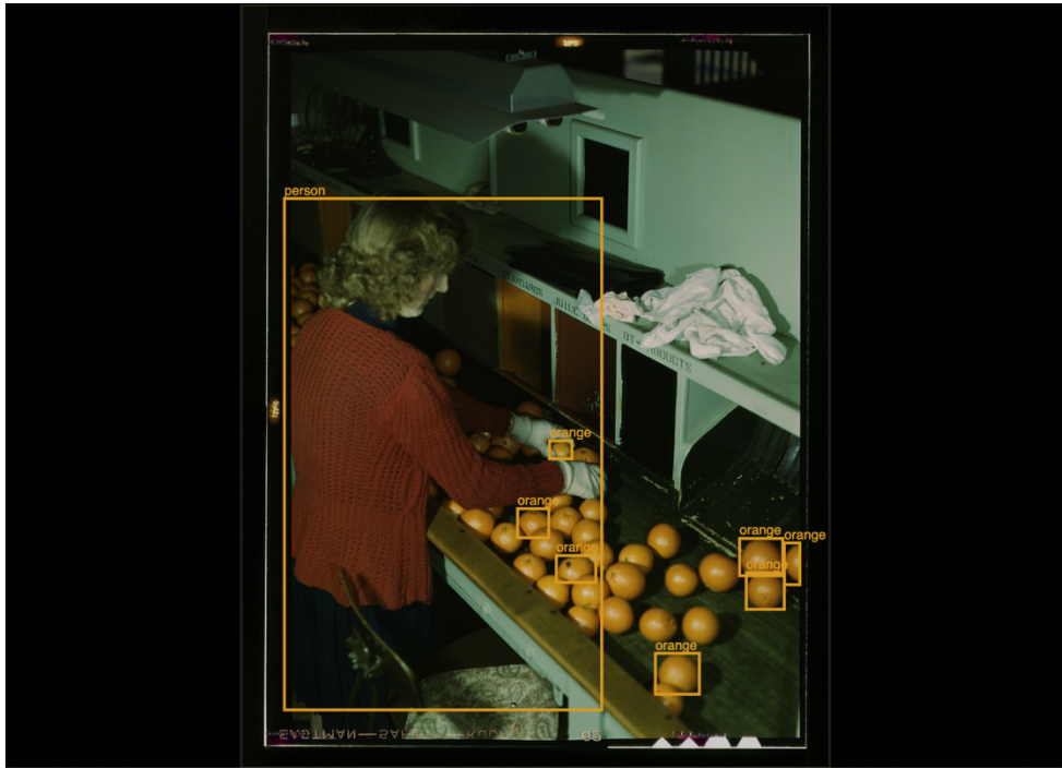
Figure 7. Object detection results on a color FSA-OWI image. It detects the person and some of the oranges, but most of the oranges are missed even when setting a very low confidence score. [2017878149]
