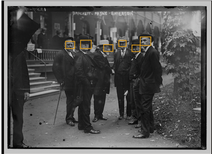
Figure 1. Example of results from a face detection algorithm, showing the ability to detect faces at different angles to the camera. [2014687262]
