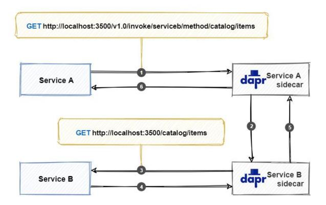
Figure 6-1. How Dapr service invocation works.
