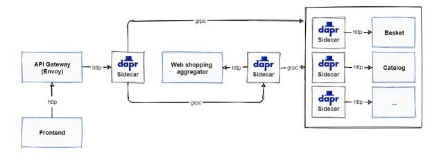
Figure 12-6. Updated eShop architecture using Dapr.
