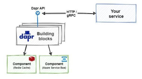
Figure 13-2. Dapr building block integration.
