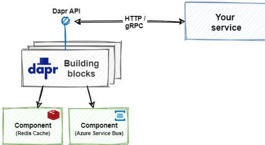
Figure 13-2. Dapr building block integration.
