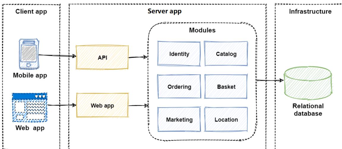
Figure 1-1. Monolithic architecture.
