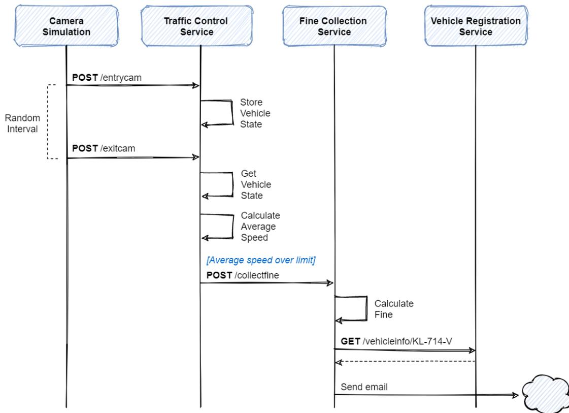
Figure 4-2. Sequence diagram of the simulation flow.
