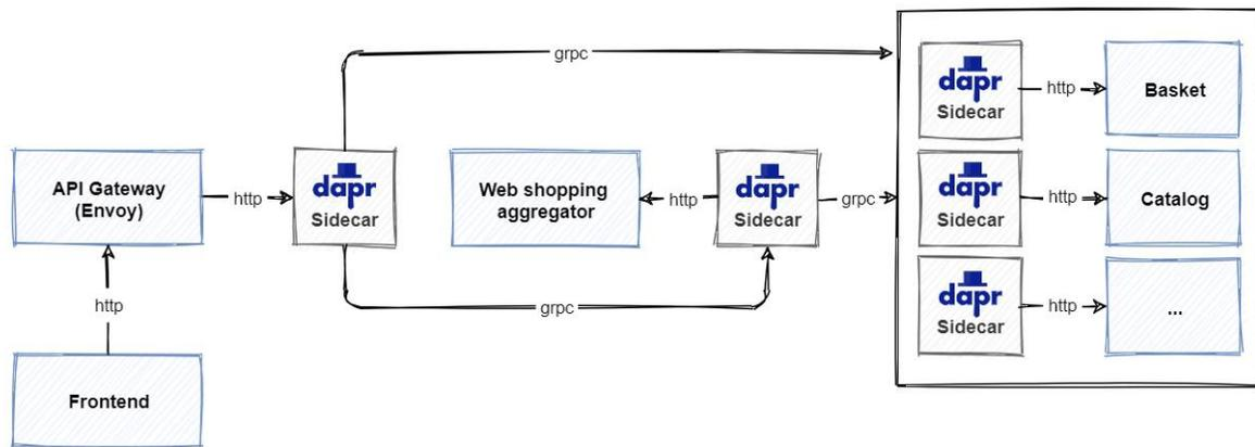
Figure 12-6. Updated eShop architecture using Dapr.
