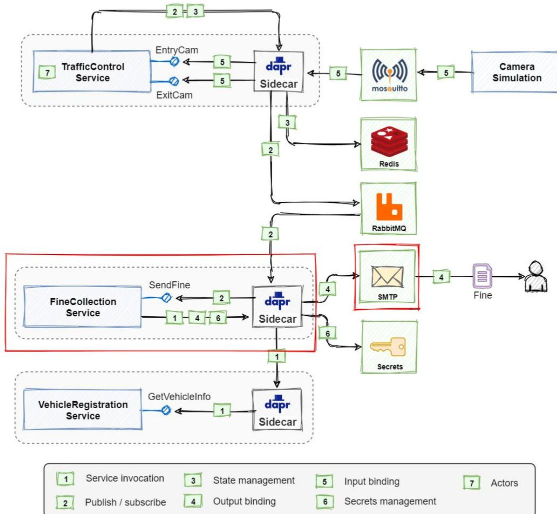
Figure 8-5. Conceptual architecture of the Dapr Traffic Control sample application.
