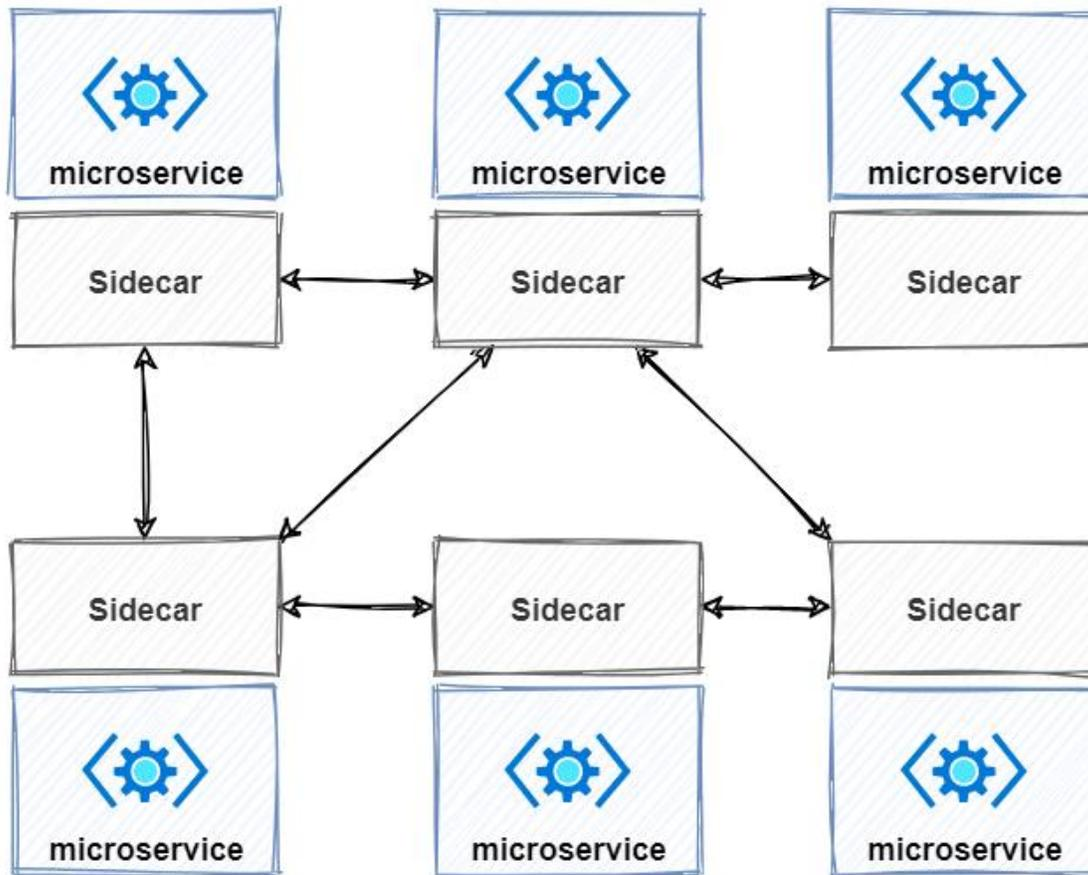
Figure 2-8. Service mesh with a side car.
