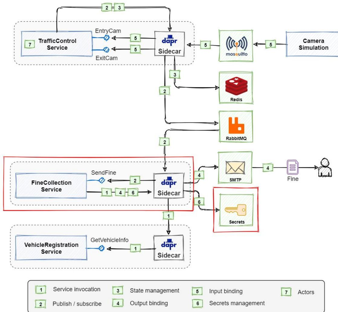
Figure 10-2. Conceptual architecture of the Dapr Traffic Control sample application.
