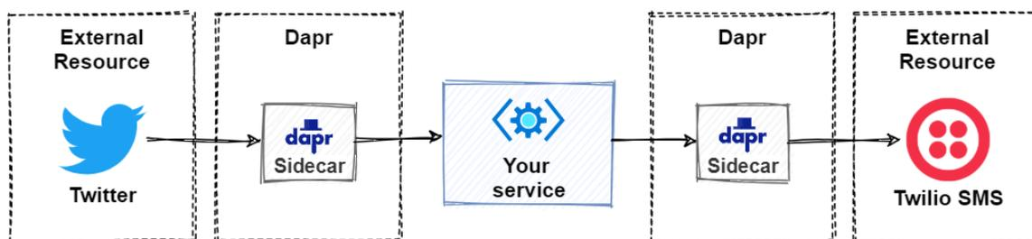
Figure 8-1. Conceptual architecture of a Dapr resource binding.
