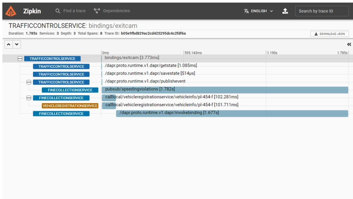
Figure 10-12. Zipkin end-to-end tracing example.
