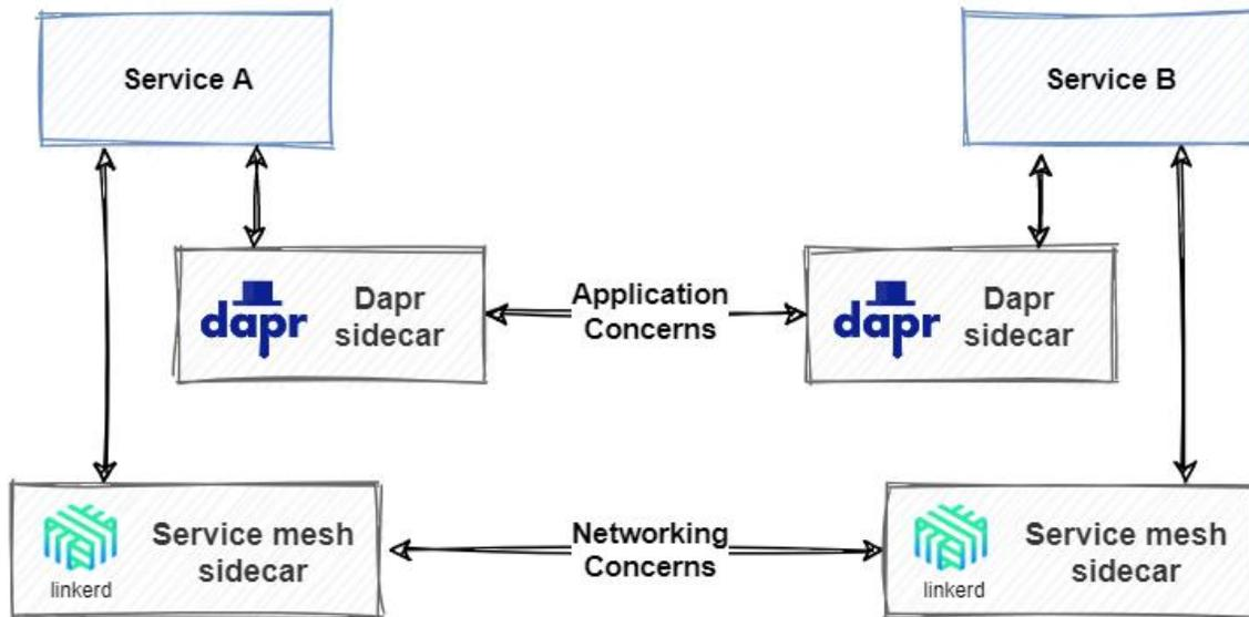
Figure 2-9. Dapr and service mesh together.
