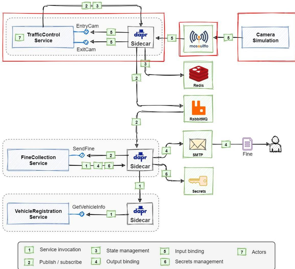
Figure 8-4. Conceptual architecture of the Dapr Traffic Control sample application.
