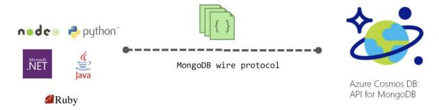
Figure 7-20. Using MongoDB API and protocol to access Azure Cosmos DB
