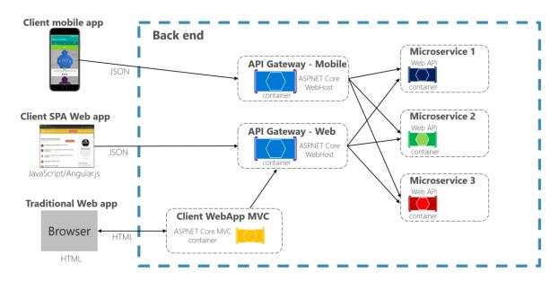
Figure 4-13.1. Using multiple custom API Gateways
