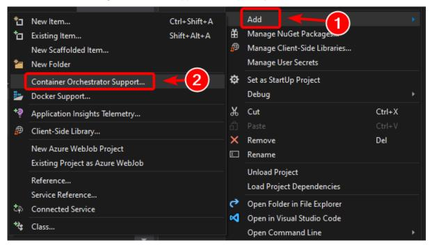
Figure 5-7. Adding Docker support in Visual Studio 2022 by right-clicking an ASP.NET Core project
