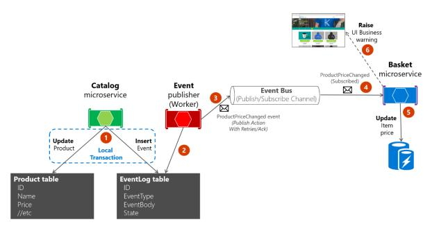
Figure 6-23. Atomicity when publishing events to the event bus with a worker microservice
