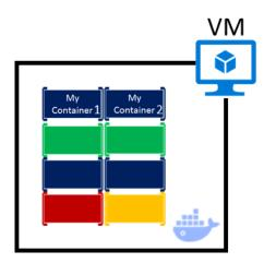
Figure 5-10. VM with Docker containers deployed
