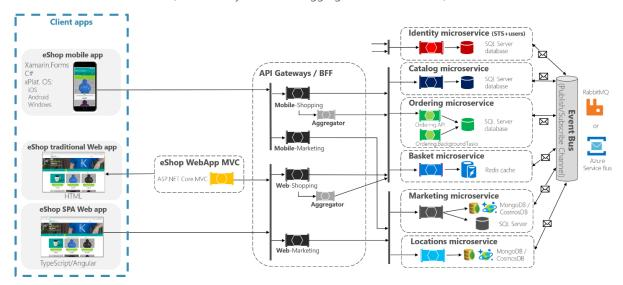
Figure 6-37. eShopOnContainers architecture with aggregator services
