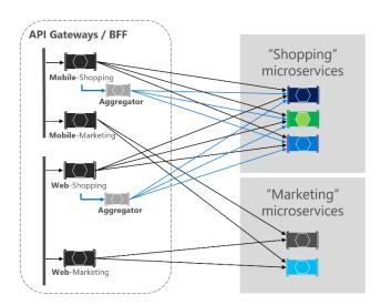
Figure 6-38. Zoom in vision of the Aggregator services
