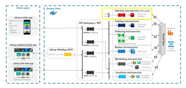
Figure 6-39. Position of the Identity service in eShopOnContainers
