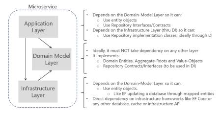
Figure 7-7. Dependencies between layers in DDD
