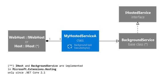
Figure 6-27. Class diagram showing the multiple classes and interfaces related to IHostedService
