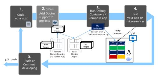
Figure 5-15. Simplified workflow when developing with Visual Studio
