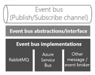
Figure 6-20. Multiple implementations of an event bus
