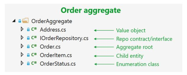
Figure 7-11. The order aggregate in Visual Studio solution
