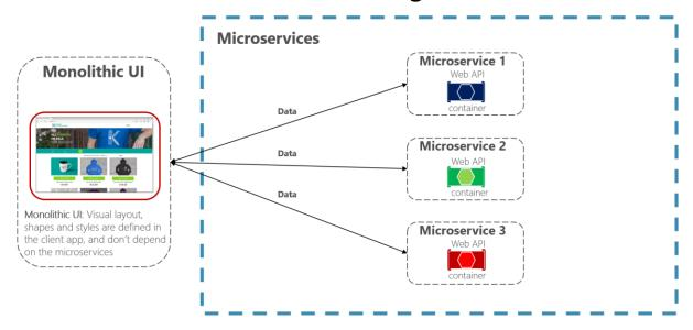
Figure 4-20. A monolithic UI application consuming back-end microservices
