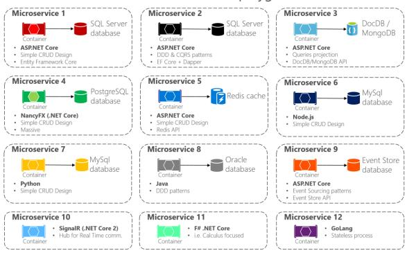
Figure 6-3. Multi-architectural patterns and the polyglot microservices world
