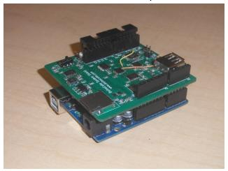
2. Stack the GFX Shield on top of the UI Shield.
