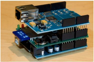
The stacking structure allows all Arduino pins to reach all pins of each shield. As long as the shields' control pins don't overlap, the Arduino board can access all of the connected shields.
