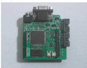
The GFX Shield contains a **field programmable gate array** (FPGA). An FPGA is a programmable logic chip. But instead of a software program, it lets you program a circuit onto it. The GFX Shield's FPGA contains a custom video and audio system called the **Core**. As the name suggests, the Core is central to the operation of DuinoCube.
