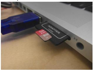
9. Insert microSD card into the microSD slot on the UI Shield. The GFX shield has been removed in the photo for visibility.
