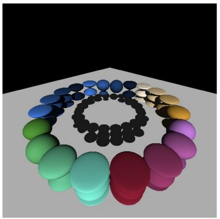
This tutorial demonstrates the creation of a dynamic scene, consisting of several deforming spheres. Half of the spheres use the RTC\_BUILD\_QUALITY\_REFIT geometry build quality, which allows Embree to use a refitting strategy for these spheres, the other half uses the RTC\_BUILD\_QUALITY\_LOW geometry build quality, causing a high performance rebuild of their spatial data structure each frame. The spheres are colored based on the ID of the hit sphere geometry.
