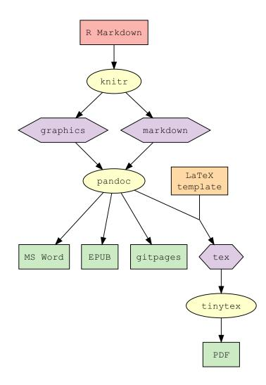
**Figure 1.** Illustration of document generation in gaelsdown, with inputs in red/orange rectangles, software in yellow ellipses, intermediate products in purple hexagons, and outputs a green rectangles.
