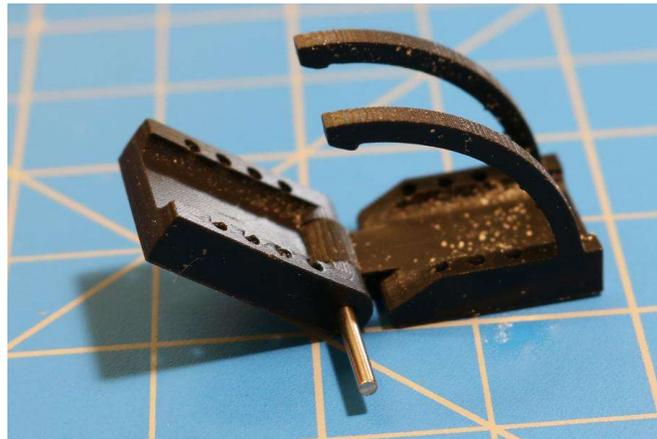
Figure 5: Pin insertion for the hinge.
