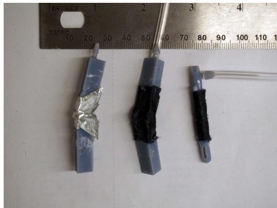
Figure 24: Images of the various legs with different joint materials. The left leg has a triangular cross section with Mylar, the middle leg has a triangular cross section with silicone impregnated cloth, and the right leg has a circular cross section with silicone impregnated cloth.
