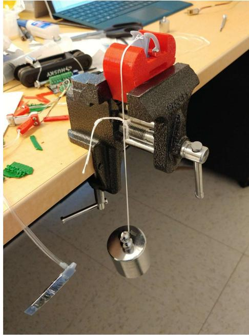
Figure 21: De-mate test with a 500g weight (4.90N).
